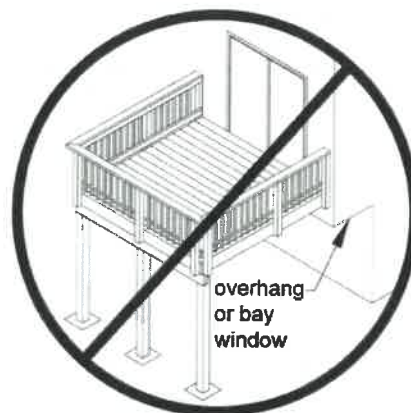
Figure 18. No Attachment to House Overhang with Ledger.
